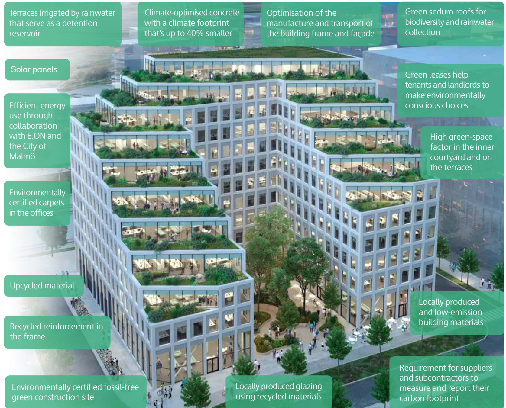
Above are some examples of the project's environmental initiatives and how we plan to meet the requirements for certification.
