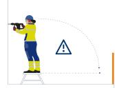
Safe distance to the edge when working from a 2-step trestle is 1.5 m. For leaning ladder or step ladder is the safety distance the same as the standing height (min. 1.5 m)
